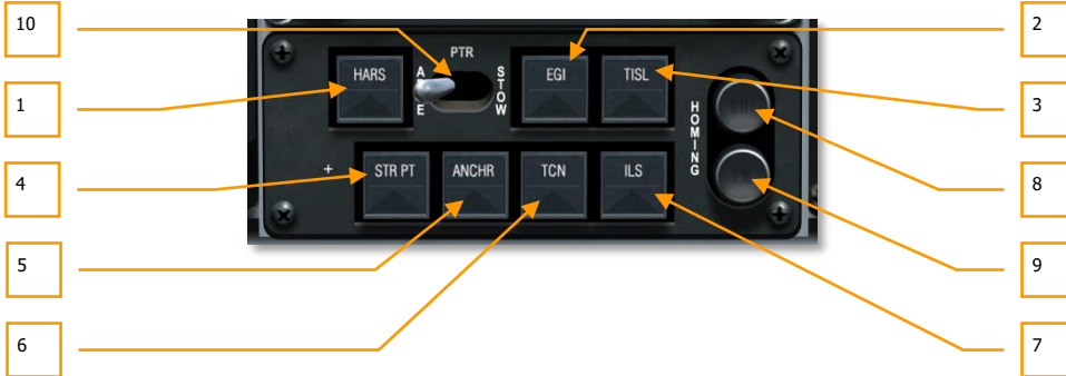
Abb. 90: Navigation Mode Select Panel (NMSP)
