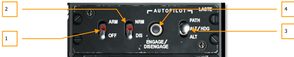
Abb. 109: LASTE Control Panel
