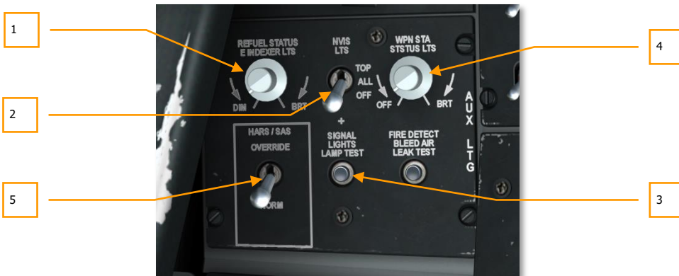
Abb. 116: Auxiliary Lighting Control Panel
