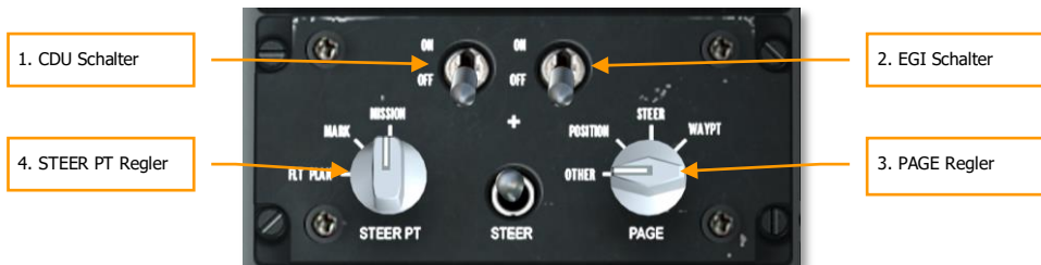
Abb. 307. Auxiliary Avionics Panel
