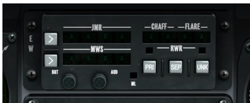
Abb. 87: Countermeasures Set Control (CMSC)
