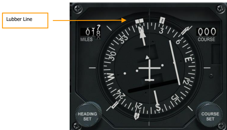
Abb. 376: Horizontal Situational Indicator (HSI)
