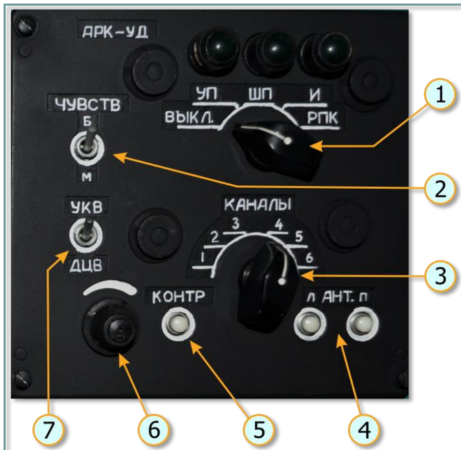
Fig. 6.17. ARK-UD control panel
