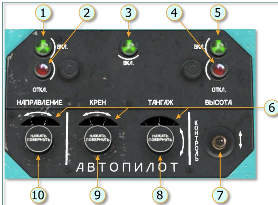
Fig. 7.44. Autopilot control panel
