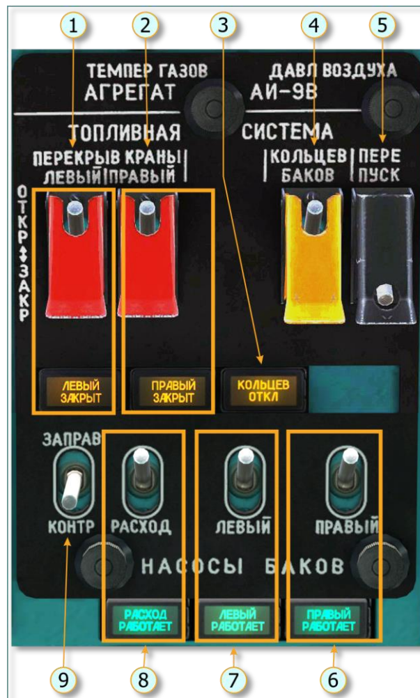
Fig. 7.7. Fuel System Control Panel, Center overhead console
