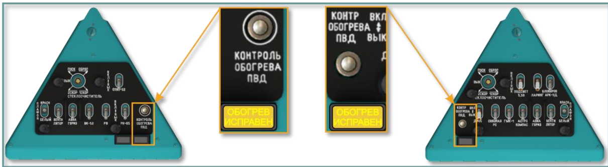
Fig. 5.38. Pitot heat test buttons and HEATER OK annunciators
