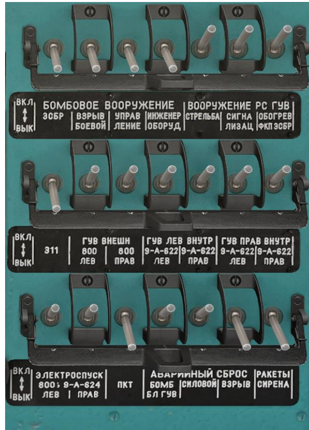
Fig. 11.3. Weapons Systems circuit-breakers.
