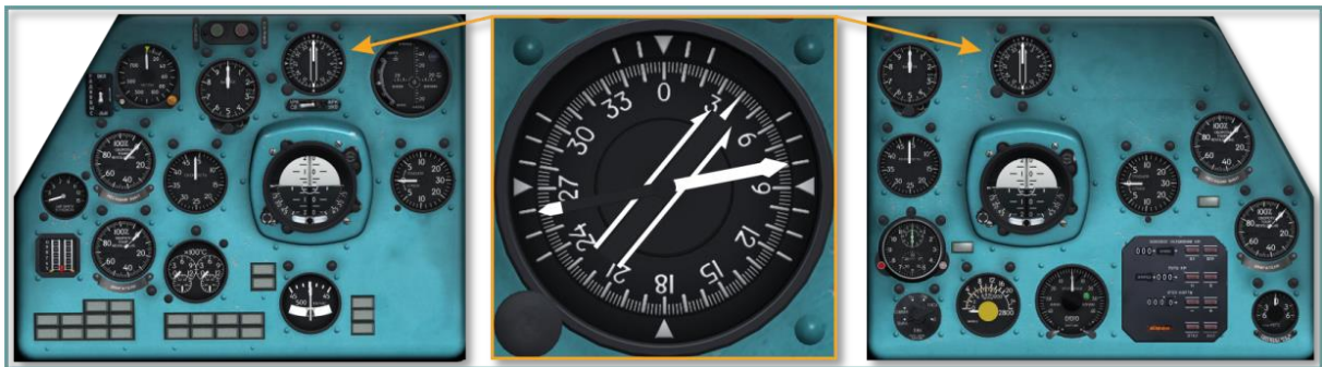
Fig. 5.49. UGR-4UK directional gyro
