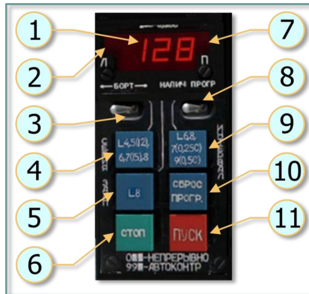
Fig. 6.24. UV-26 control panel:
