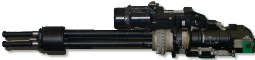
Fig. 11.23. GShG-7.62 7.62 mm 4-barrel Gatling gun
