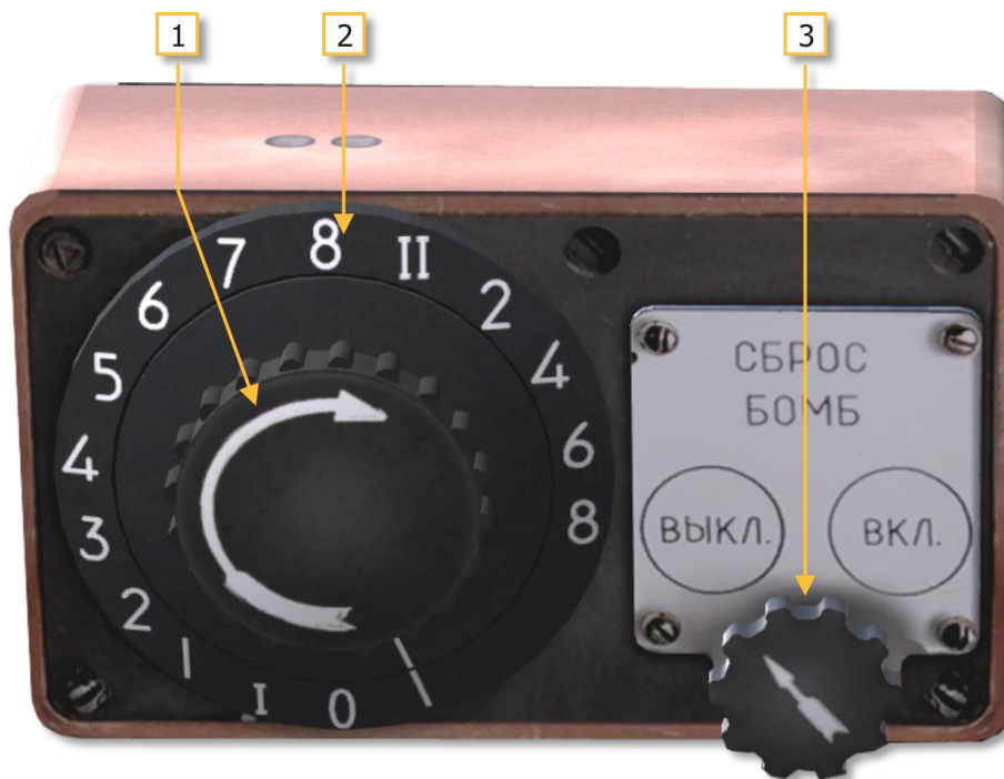
Fig. 11.8. ESBR control box
