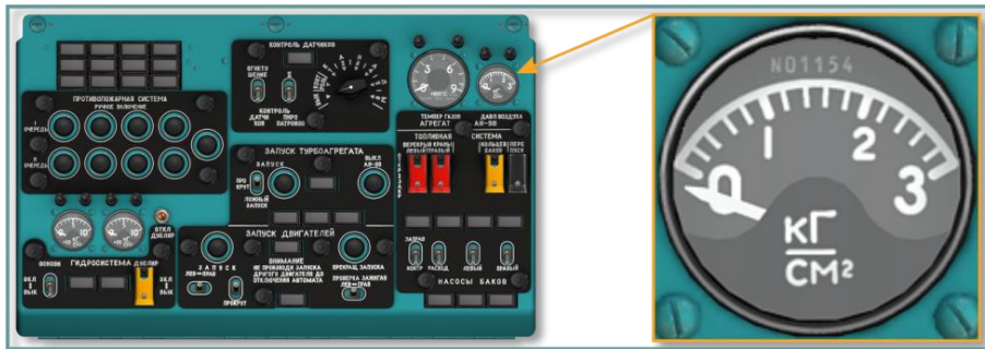
Fig. 5.29. APU air pressure gauge, center overhead console
