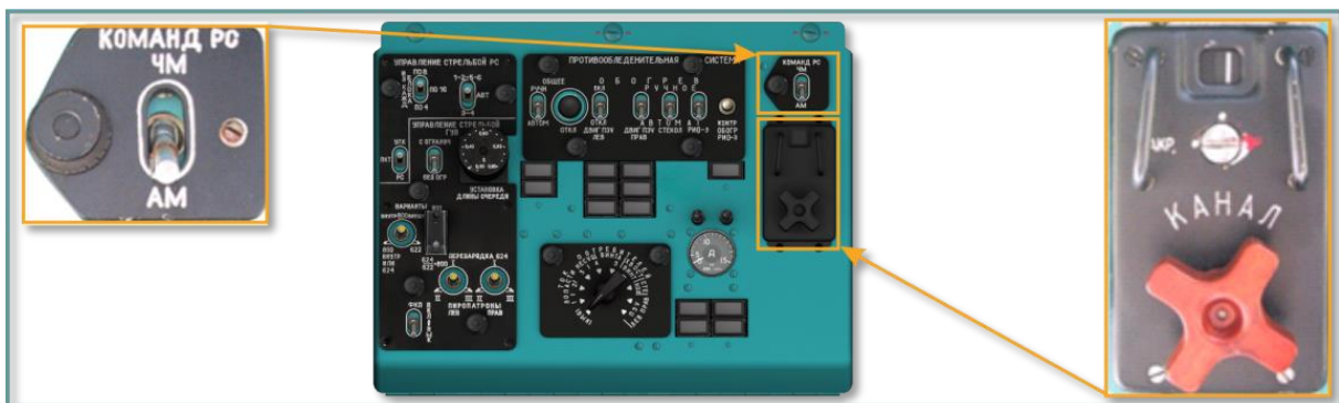
Fig. 6.2. Left overhead console: R-863 "КОМАНД. РС АМ-ЧМ" (AM-FM) switch (FM up position, AM down position); R-863 "КАНАЛ" (CHANNEL) selector panel with 20 available channels
