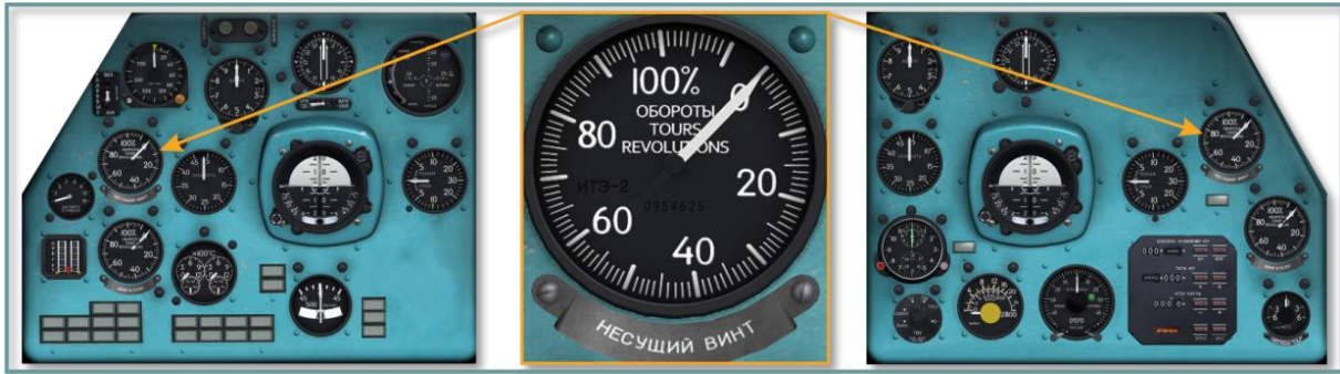
Fig. 5.21. Pilot's and copilot's main rotor tachometers
