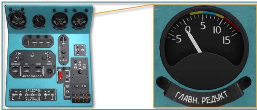
Fig. 5.26. Main transmission oil temp gauge, center console
