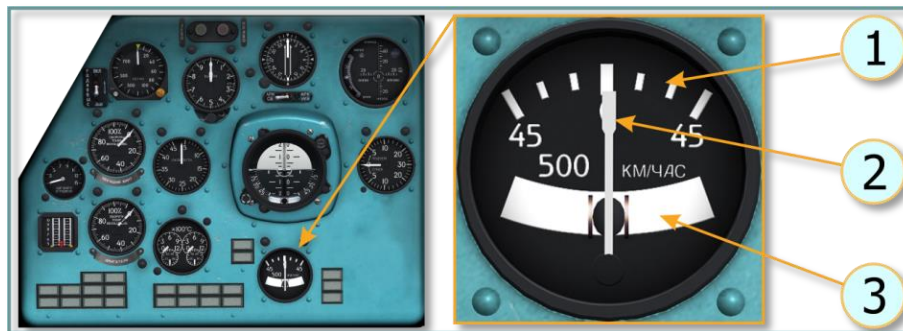
Fig. 5.46. Turn and slip indicator
