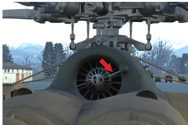
Fig. 7.19. Radioisotopic Ice Detector
