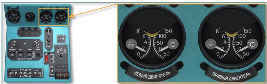
Fig. 5.22. Oil pressure/temperature gauges, center console
