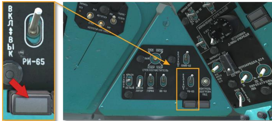
Fig. 6.11. Switch and warning annunciator "ВКЛЮЧИ РИ-65" (TURN ON RI-65) on the left triangular panel
