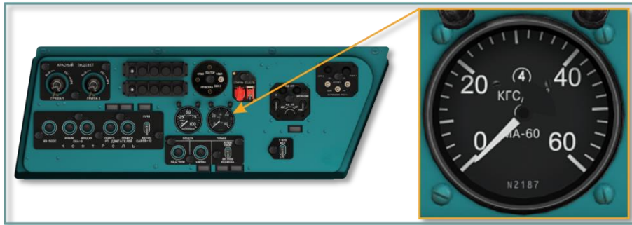
Fig. 5.35. Brake pressure gauge, left side panel
