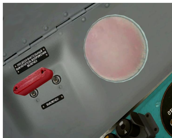
Fig. 11.4. The Master Arm switch and its associated red caution lamp.
