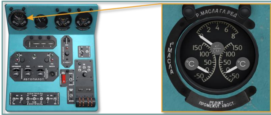
Fig. 5.23. Three pointer drive system oil pressure/temperature gauge, center console
