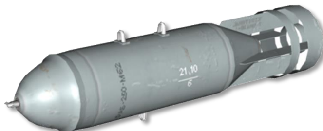
Fig. 11.26. FAB-250 250 kg free-fall bomb
