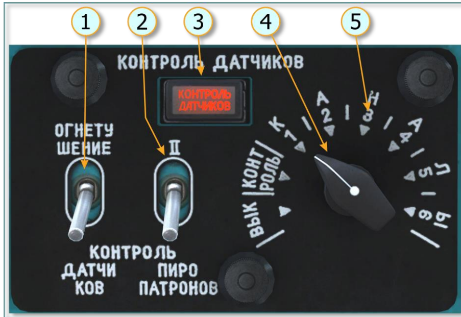
Fig. 7.29. КОНТРОЛЬ ДАТЧИКОВ (MONITORING OF SIGNAL DEVICES) Center overhead console
