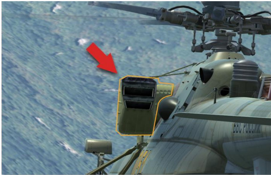
Fig. 7.49. Exhaust IR suppression devices
