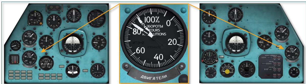
Fig. 5.20. Pilot's and copilot's dual engine tachometers
