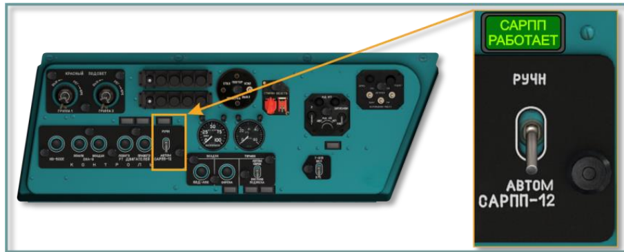
Fig. 7.40. SARPP-12D1M FDR power switch and indicator light, left side panel
