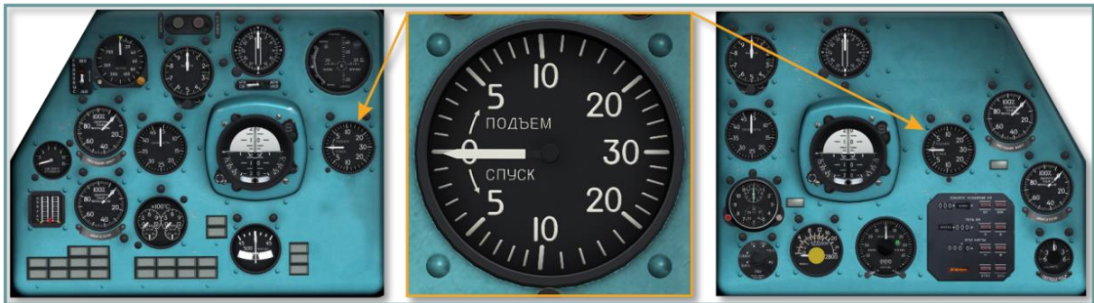
Fig. 5.43. Vertical speed indicator (VSI)
