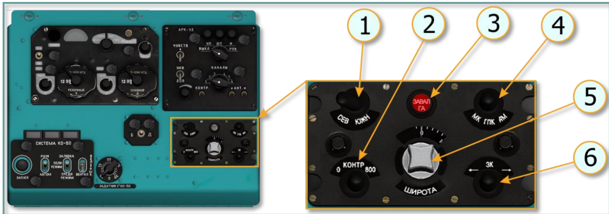
Fig. 5.48. PU-26 control panel, right overhead console
