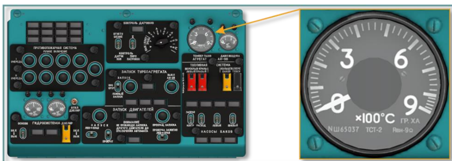
Fig. 5.28. APU EGT gauge, center overhead console
