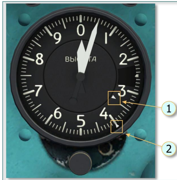
Fig. 5.42. Setting helipad altitude using adjustment knob
