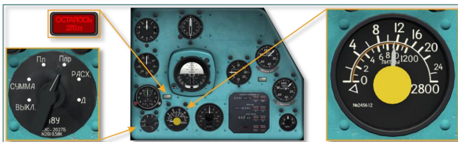
Fig. 5.32. Fuel quantity gauge
