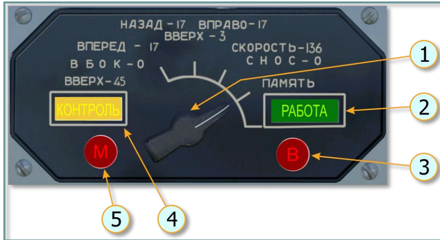
Fig. 6.18. Doppler control panel
