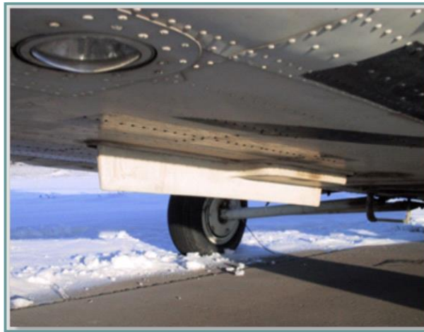
Fig. 6.13. Loop antenna and nondirectional antenna
