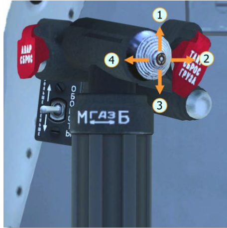
Fig. 7.36. Search/taxi light beam controls
