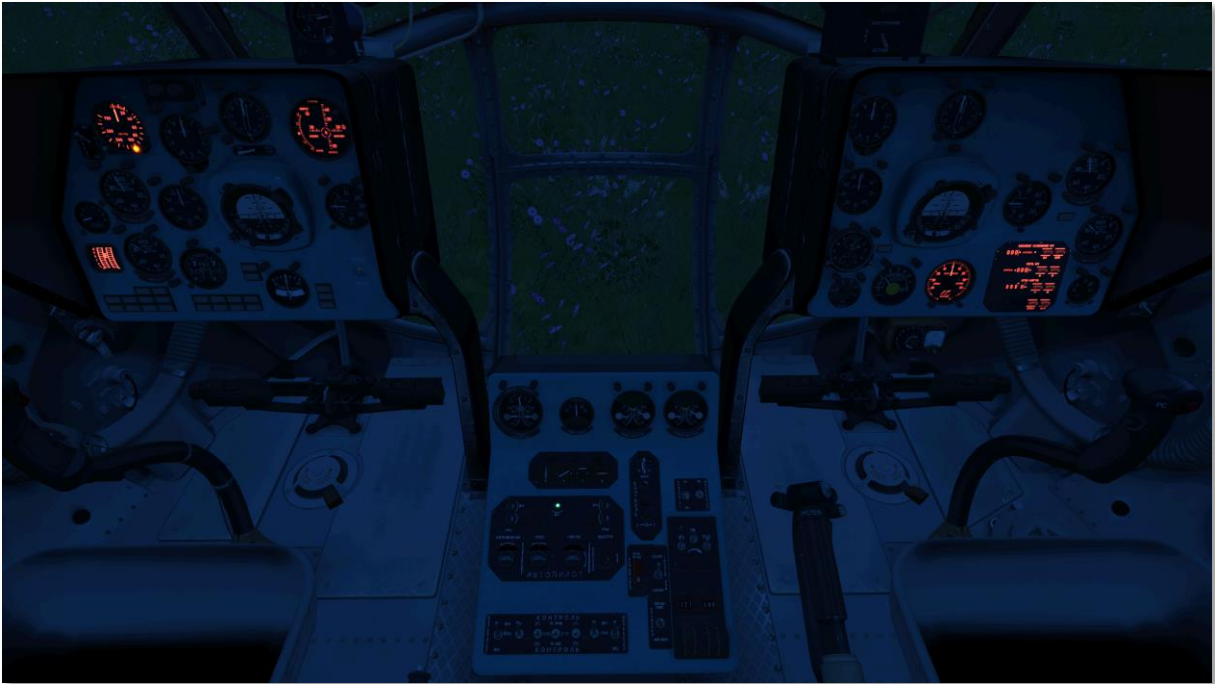
Fig. 7.38. Instruments backlit by the "Подсвет 5,5V" (Backlight 5.5V) system
