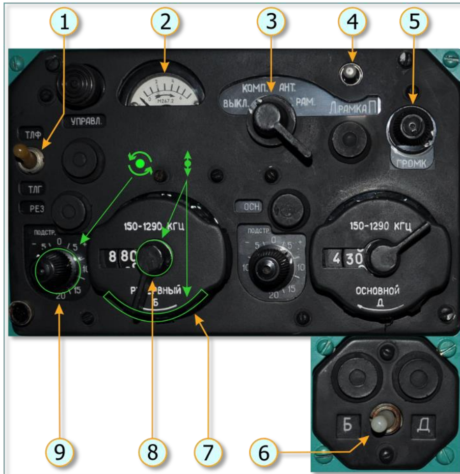
Fig. 6.14. ARK-9 control panel
