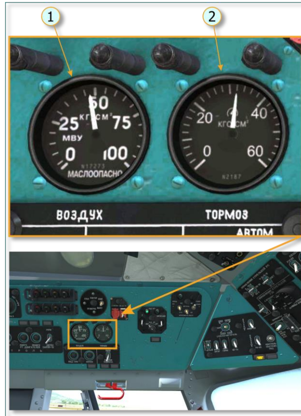
Fig. 7.23. Pressure gauges of Pneumatic System
