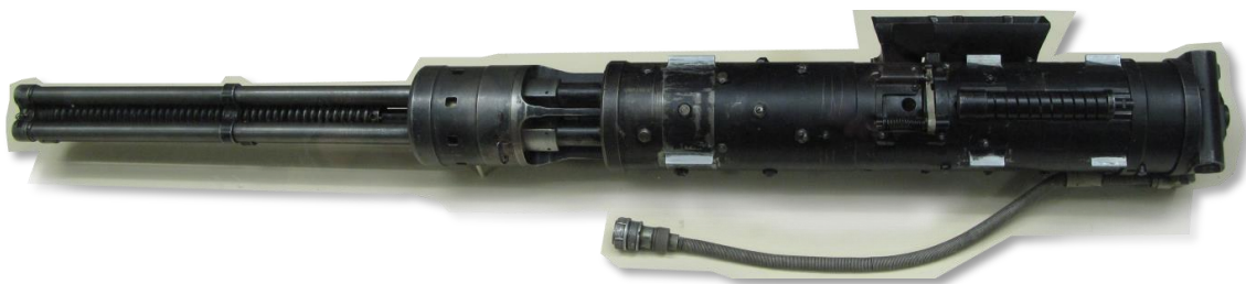
Fig. 11.22. YakB-12.7 12.7 mm 4-barrel Gatling gun
